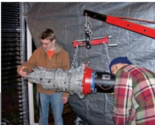
The 100 hp DC motor bolted to the original transmission.
